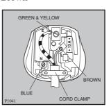
The wire coloured green and yellow must be connected to the terminal marked with the letter «E» or by the earth symbol  $\perp$  or coloured green and yellow.
